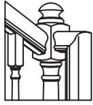
The following instructions are designed to be used for the installation of LJ-4091 Box Newels using the L.J. Smith LJ-4091MTG Box Newel Mounting Kit. These instructions assume the location of each box newel has already been marked on the stairway and balcony.
